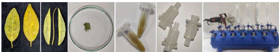
Figure 3. Laboratory procedures adopted to extract pathogen DNA from suspected leaf samples using the wizard column method
